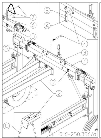
Carry out this operation very carefully and with suitable lifting equipment because the drawbar 2 is heavy and bulky. Weight 170kg/375lbs. First of all remove the nut A and packing retainer B from the crosspiece assembly 1. The nuts A and packing retainers B will not be reused. To work safely and make the next assembly easier, set the drawbar 27 on a support C.
