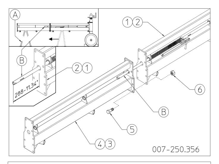
Check that pipe B protrudes about 288mm-11.34" from section 1-2. Note: this measurement is with the cylinder to which it is attached completely closed, and the total pipe length must be 1670 mm - 65.75".
