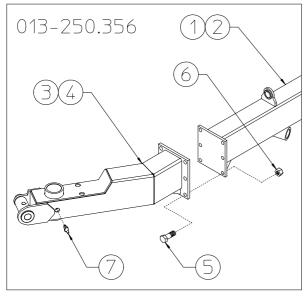
Attach the wheel supports 3-4 to sections 1-2 (RH-LH) using bolts 5 and nuts 6.
