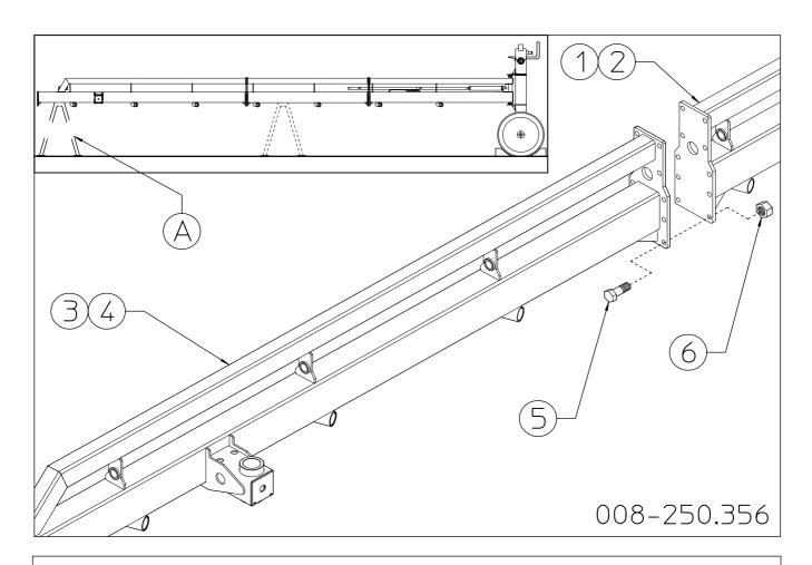
Now attach sections 3-4 (RH-LH – 105kg/230lbs) to sections 1-2 (RH-LH) using bolts 5 and nuts 6.
