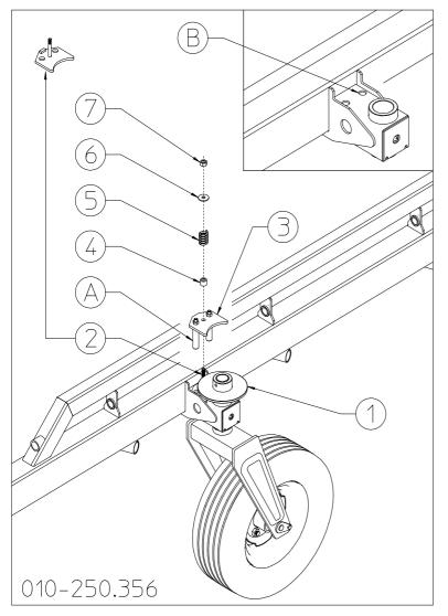
Attach the plate with bolt 2 underneath flange 1. Attach the counterplate 3 over flange 1, inserting the counterplate pins A into the holes in the plate with bolt 2 and into holes B in the sections. Place the bushing 4, spring 5 and washer 6 over the plate 2 bolt and put nut 7 on the bolt.
