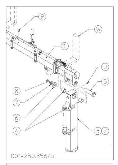
Insert bushings 4 in the openings in supports 2-3 (RH/LH - 40kg/88lbs). Lift unit 1 (weight 110kg/245lbs) with a suitable forklift W. Connect the vertical supports 2-3 to the crosspiece assembly 1 using pin 5, washers 6-7 and bolt 8.
