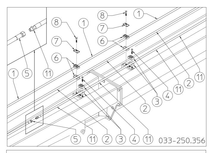
Continue to secure hose 11 with collars 3 and screws 4. Continue to secure hoses 1-2 with collars 6, clamps 7 and bolts 8.
