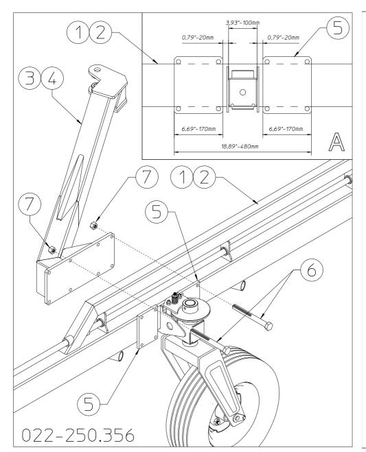
Attach the opening arms 3-4 (RH-LH) to sections 1-2 by of the means counterplates 5, bolts 6 and nuts 7. In box Α the theoretic measurements are for given the assembly of arms 3-4 and counterplates 5. At this stage do not fully tighten nuts 7, because when the cylinders are attached (see step 27) it may be necessary to move the arms 3-4 and counterplates slightly forward or backward to allow the correct installation of the cylinders.
