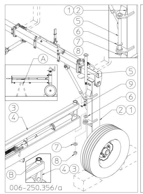
Check that manufacturer has assembled on the vertical supports 1-2 (RH-LH) the pins 5, spacers 6, washers 7 and nuts 8 that you will use for assembly in the order in which you find them assembled.
