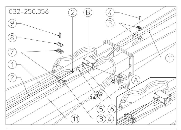
Send hose 11 under bracket A and continue to secure it with collars 3 and screws 4. Apply washer 6 and nipple 5 to hole B on the flow divider. Bring the female end of hose 2 near the nipple and extend it along drawbar C toward the front of the machine parallel to hose 1 already assembled. Connect the female end of hose 2 to the nipple 5 without fastening completely.
