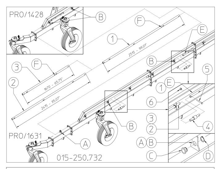
Check to make sure the manufacturer has correctly secured the bushings C with retaining rings D on all the RH and LH sections.
