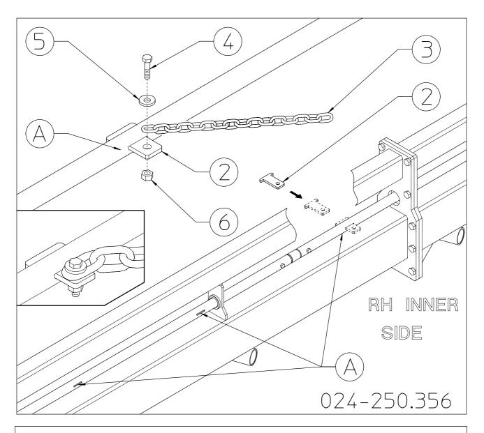
Insert brackets 2 in the slots A in all the pipes (RH-LH). Attach the chain 3 at all the brackets 2 using the bolt, washer 5 and nut 6.
