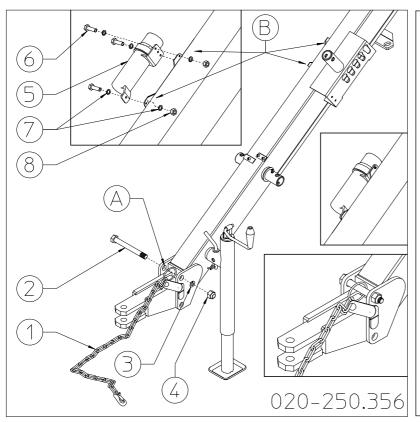
Attach the safety chain 1 to the holes A in the drawbar using the bolt 2, washer 3 and nut 4.
