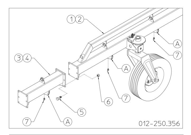
Note: Sections 3-4 (RH-LH) are to be assembled only for MKE-PRO/1631. Attach sections 3-4 (RH-LH) to sections 1-2 (RH-LH) using bolts 5 and nuts 6. Note: For MKE-PRO/1428 and MKE-PRO/1631 — At this point the assembly of the sections is completed. Apply the grease nipples 7 to all the bushings A on all the RH and LH sections.
