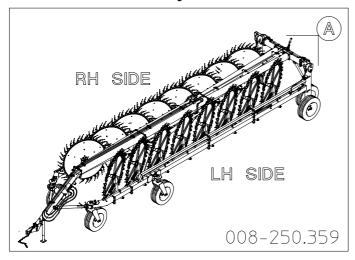
As regards the indicating of right/left, they are understood to be attributed observing the machine from point A (behind the machine) looking forward.
