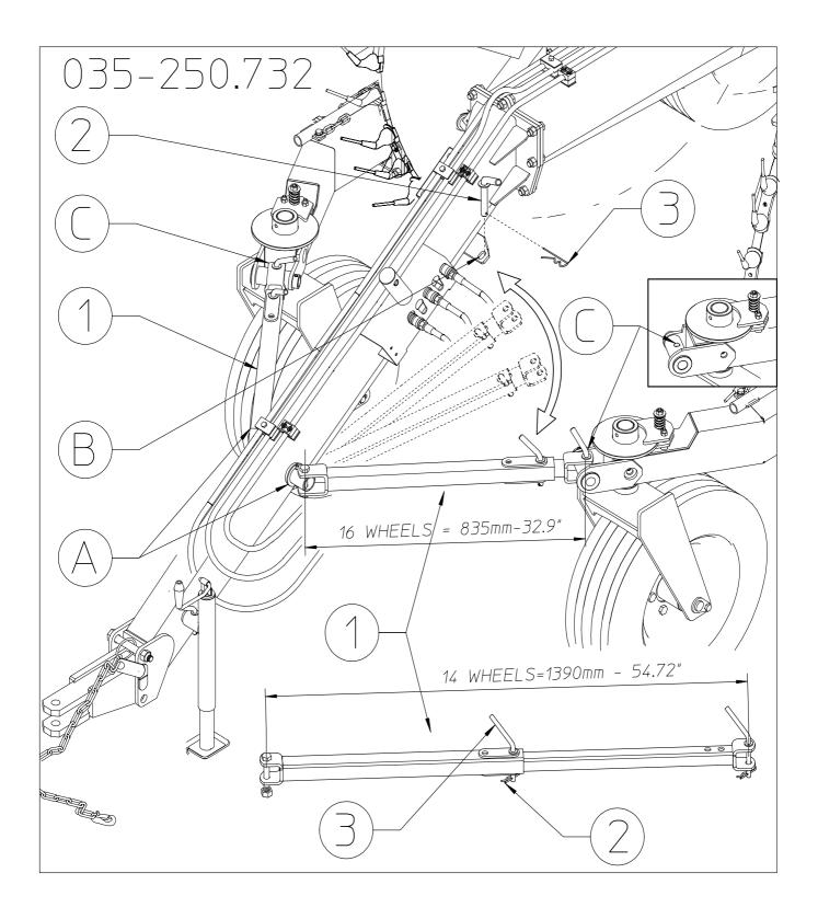
The assembly is now completed. The machine is ready to be lubricated and then used. If for lubricating or for other reasons the machine must be moved, the safety arms must be rotated from the working position A-B to the transport position A-C. To do this you must remove the pin 2 and clip 3 from position B, rotate the arm until it reaches position C, and then fasten it again with pin 2 and clip 3.
