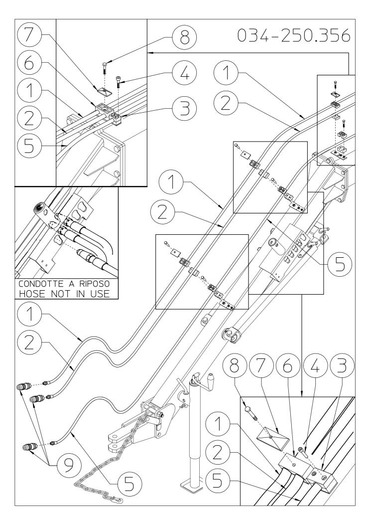
Continue to secure hose 5 with collars 3 and screws 4. Continue to secure hoses 1-2 with collars 6, clamps 7 and bolts 8.
