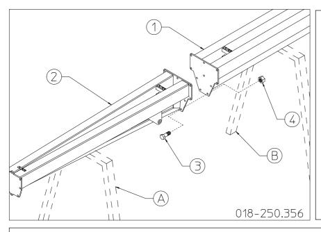
Carry out this operation very carefully and with suitable lifting equipment because the drawbar 2 is heavy and bulky. Weight 135kg/297lbs plus the preceding drawbar.
